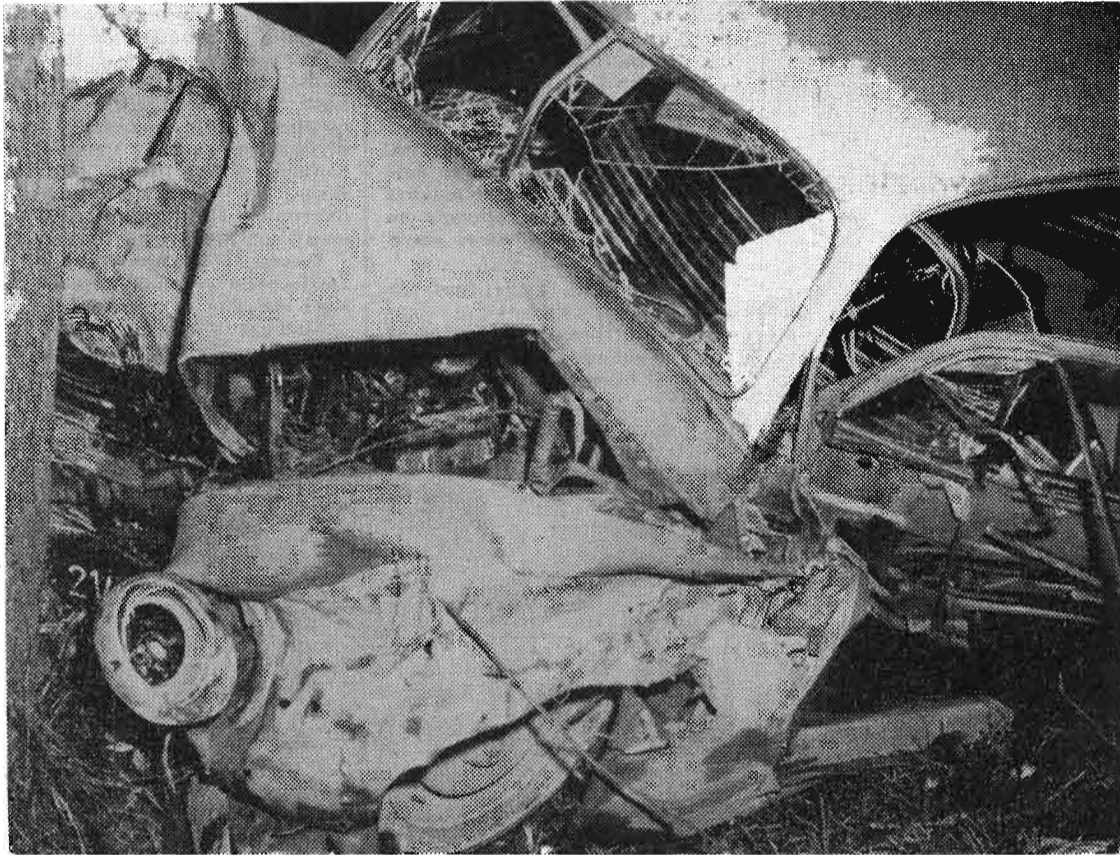
Twisted steel and broken glass bare mute evidence as to what can happen when a car traveling 60 miles per hour (or 88' per second) meets a tree head-on. An appropriate likeness would be to drive your auto off the roof of a 12 story building — the impact is approximately the same.
